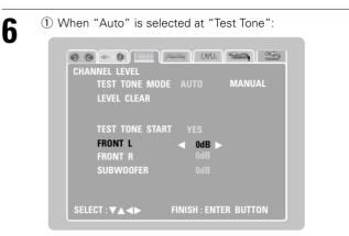
Test tones are automatically output from the speakers at intervals of 4 seconds for two of the cycles shown below, then at intervals of 2 seconds from the third cycle on.
